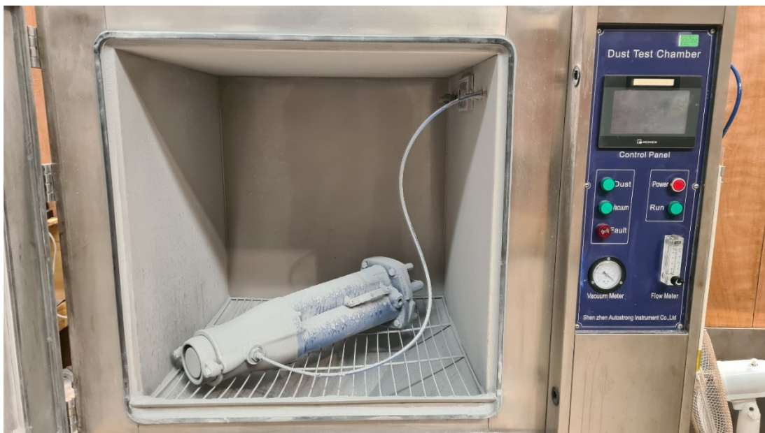
Picture 2 Coupler in dust test
